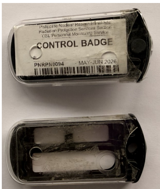
Figure 2: Damaged cases in service
