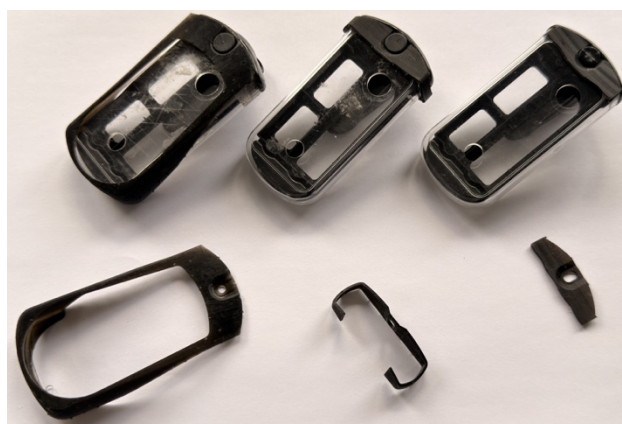
Figure 3: Repaired Dosimeters (Above) and Implemented parts (Below)
